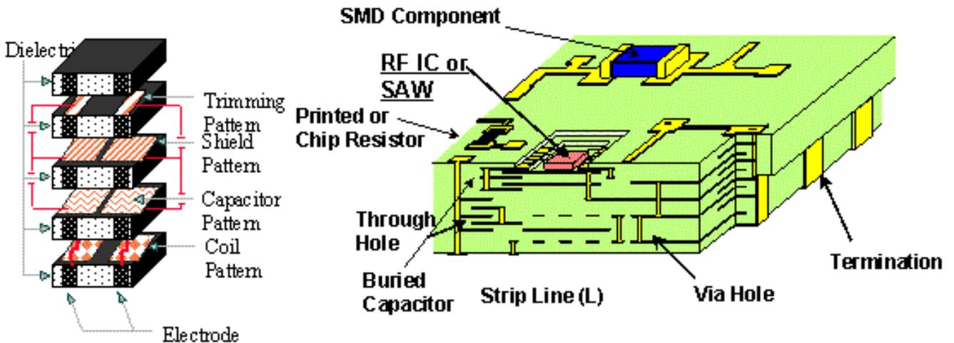
**Example of LC Filter LTCC structure.** Chip sizes ranging from 2mm x 1.25mm up to 3.2mm x 1.6mm.
